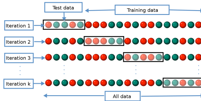
Slika 1. Shema križne validacije (Izvor: https://en.wikipedia.org/wiki/Cross-validation_(statistics)#/media/File:K-fold_cross_validation_EN.svg )
