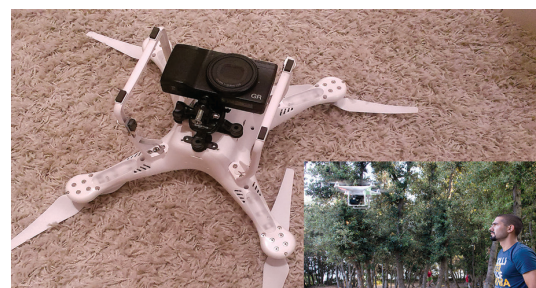
Figure 1: Dji Phantom2 mounted with a RicohGR compact digital camera, author: M. Vuković; Lower right corner - UAV mid-flight, author: M. Doneus
